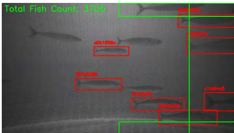
Figure 16. Automated tracking of mackerel imaged with an in-trawl camera system.
