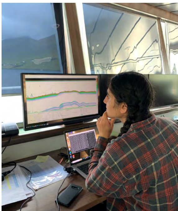
Figure 31. Taraneh using echosounders to look at biological organisms in the water column.
