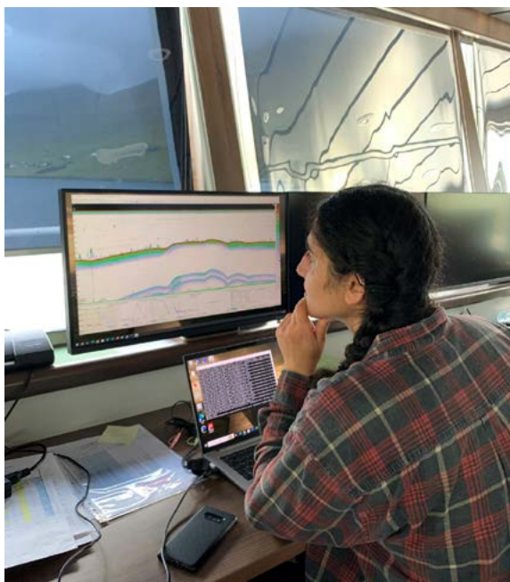
Figure 23. Taraneh using echosounders to look at biological organisms in the water column.
