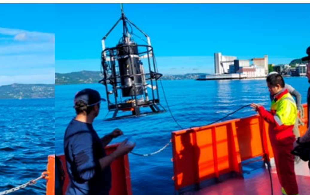
Figure 8. An acoustic probe with 5 echo sounders was used to do experimental measurements on calibration spheres at Sandvikflaket just outside Bergen. Backscatter from two calibration spheres positioned above each other with different separation distance.
